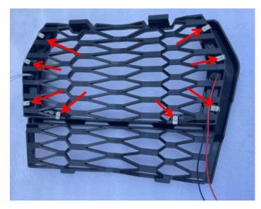
3. Install the front mesh grill to the vehicle, then unplug the headlight wiring harness plug-ins of the original vehicle, connect the headlight wiring harness to the plug-in of the accent light, and connect the other end to the wiring harness plug-in of the vehicle, as shown in the picture:
