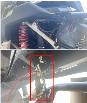
8. Connect the remaining harness of the #2 adapter wire to the rear bar light harness, and then secure the rear accent light to the vehicle with screws.
