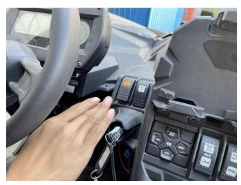
7. Prepare the #2 adapter cable, connect the extension cable to the #2 adapter cable (use the connection method in step 6. (Black wire connected to black, red wire connected to red), the vehicle rear tail light harness plug-in disconnected, with 2 adapter wire corresponding to the harness plug-in and tail lights and the entire vehicle harness reconnected.
