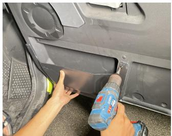
2. Drill a screw hole by a 3MM drill bit as indicated in the picture, and then tighten the screw. (The storage box on the other side can be installed as the same steps 1-2) As shown in the picture:
