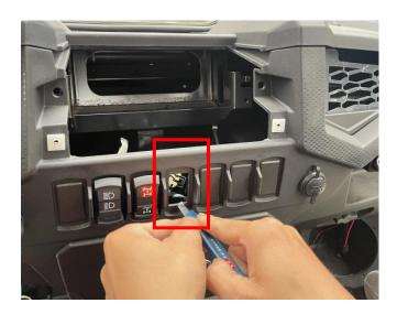
2. Prepare the No. 1 converter cable in the product, and insert the end with the transparent sheath into the switch lugs (note the wiring position). Pass the converter cable through the switch hole, and then install the switch. As shown in figure:
