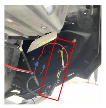
6. Connect the rear accent light harness to the No.2 conversion cable, and then place the rear accent light on the top of the rear bumper of original vehicle, and then fix the both sides of light with screws. As shown in figure:
