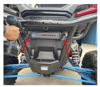
7. After completing above steps, return to the cab, thread the No.1 conversion cable with the connection coil out of the cab to the binding post through the outlet hole, and then install the instrument storage box. As shown in figure:
