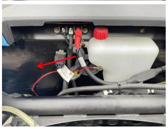
8. Unscrew the nuts of the positive and negative terminals on the binding post, cover the copper pieces of the No.1 conversion cable on the binding post according to the positions of the positive and negative terminals (black wire cover the black one, red wire cover the red one), then screw the nuts, and finally reinstall the vehicle cover. As shown in figure:
