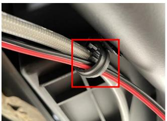
5. Connect the extension cable to the No. 2 conversion cable, using the wiring method in Step 2, and then pull the wiring harness to the rear taillight (the loose extension cable in the middle can be fixed with cable ties), disconnect the wiring harness plug-ins of the original taillight, and reconnect the taillight and the whole vehicle with the corresponding plug-ins of the conversion cable. As shown in figure: Note: Black wire to black wire, red wire to red
