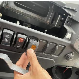
3. Open the cover of the original vehicle, get the extension cable from the accessories package and thread it through the outlet hole at the bottom of the terminal post into the vehicle, pull it to the place of the switch, and connect it with the No. 1 transfer wire (peel off the outer skin of the wiring harness joint, expose the copper wire inside, wrap the copper wire of the two wires together, and then make the insulation protection). As shown in figure:
