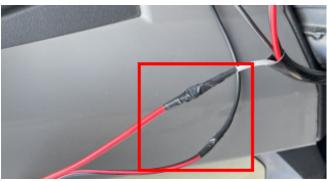
4. Extend the remaining extension cable through the gap of the vehicle body to the bottom of the vehicle. Remove the front and rear guard plates under the vehicle, and then pass the extension cable through the wire hole of the vehicle wire harness until the position of the rear wheel of the vehicle. After the wire harness was passed, the lower guard plate can be installed back. As shown in figure:
