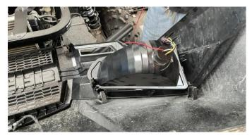
4.After installing the headlight, take out the transfer wiring in the accessories package, and connect one end with the headlight wiring harness. The other end is connected with the original wiring harness on the vehicle, as shown in the figure;
