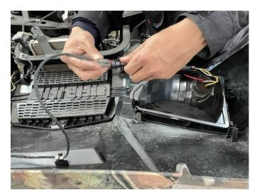
5.After connecting the headlight wiring harness, take out the white wiring harness in the accessories package, peel off the outer skin of one end, expose the copper wire, and connect it to the
