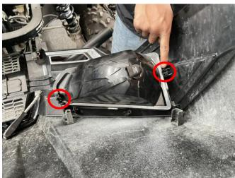
3.Place the removed steel clip to the new headlight following the position of the original headlight, and then install the light to the vehicle, and fix the screws, and the O-rings are also installed back to the original position, as shown in the picture:
