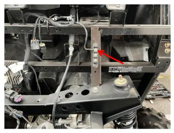
6.Pull the white wire to the position of the headlight, peel off the middle of the wiring harness(don't cut the copper wire inside), connect it with the red wire on the headlight, and complete the insulation measures, then connect the extra white wire to the red wire of the other headlight, (replace the other side headlight as above steps 2-4, as shown in figure)
