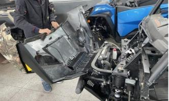
2. Firstly, remove the wiring harness plug-ins of the original headlight and remove the headlight (there is a steel clip and two O shaped rings on the headlight, remove them for later use) as shown in the figure:
