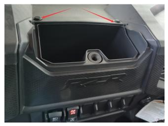
3. Take the white clip out of the hardware package, and attach it to the dashboard as illustrated below.
