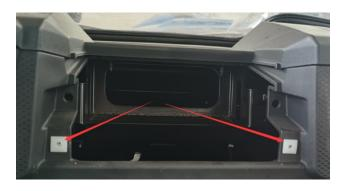
4. Fix the top of the device holder with plastic buckles as the upper red arrow positions, and fix the bottom of the device holder with screws as the lower red arrow positions.
