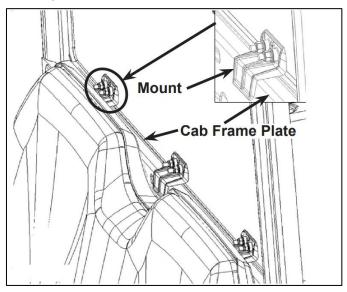
5. After installation of the rear panel, turn the handles up again to clamp the panel fully on ROPS plate.
