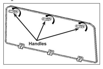
3. Push the rear panel assembly onto the ROPS.
