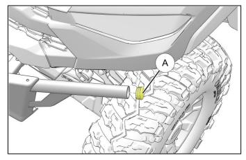
3. Loosely install threaded mount (7) to tapered fitting on LH upper bumper (1) using
