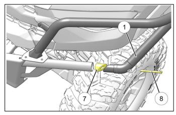
NOTICE: Over-tightening screw will prevent new bumper from entering tube opening in existing bumper.
