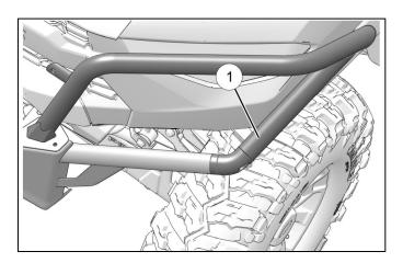
5. Loosely install LH upper bumper (1) to existing lower bumper using two screws (5) and backing plate (6).
