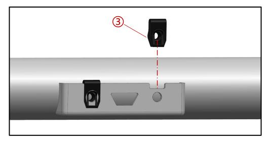
4. Align rearview mirror mount ① with U-clips ③ and install with two screws ②.
