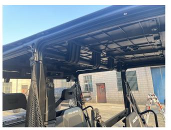
4. Take out the square pipe support rods from the accessories package, install the support rods on the roof of the rear seats, and secure both ends of the support rods with clamps. As shown in picture:
