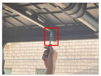
5. Fix the 6 plastic supports in the product accessories along the original roof frame (one left and one right support in the front row and two left and two right supports in the back row). Finally, the tail of the roof should be fixed with screws. As shown in picture:
