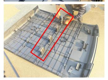
3. After completing the above steps, flip the roof to the front side, and reinforce the edges on both sides of the front side with screws, then install the roof on the original vehicle. (During installation, the 3 limit buckles on the roof need to be respectively inserted into the notch on the
