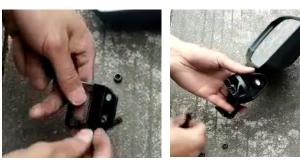
3. Install the mirror assembly to the ROPS, then tighten the screws.
