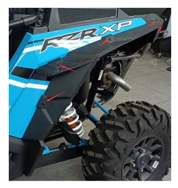
2. Repeat the Step 1 for removal of rear right fender flare on the opposite side of the vehicle.
