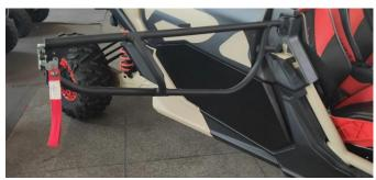
4. Fasten the M6 U-shaped clip, and fix the aluminum door at the position shown in the figure with three M6\*40 hexagon socket screws, three M6 flat washers and three M6 locknuts.
