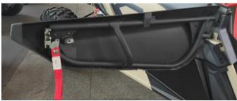
3. Remove the three groups of screws and nuts shown in the figure and the rivets at the lower end, and take down the upper half door.
