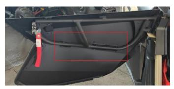
5. Fix the upper end of the aluminum door at the position shown in the figure with two M6 \* 16 socket head cap screws, two M6 flat washers and one M6 nut with washer.
