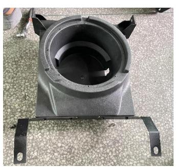
4. Remove the driver's seat, the original audio support is also removed.
