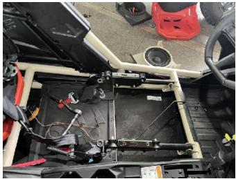
5. Unscrew the fixing nuts of the seat slide bar brackets on both sides, pull up the slide bar brackets, place the audio brackets at the installation position, and then put the iron brackets on the audio brackets on the screw posts of the seat slide bar respectively, and then press the slide bar brackets to screw back the nuts.
