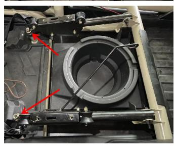
6. Use the screws in the product accessories package to fix the other side of the audio bracket, and then install the seat back to its original position.
