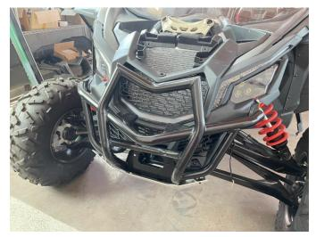
3. After removing the mesh grille and radiator deflector, replace the new radiator deflector, then put back the mesh grille, and finally put back the front bumper trim panel.
