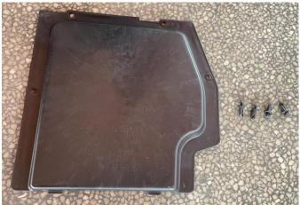
3. Adjust the front passenger seat of the vehicle to the front to facilitate the installation of the cover. Insert the two limit cards on the cover into the slot of the battery box, and then use the nylon expansion screws in the product accessories package to fix it.
