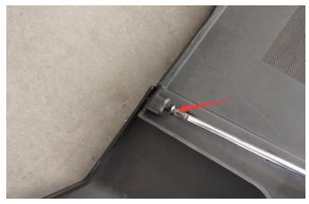
2. Fix the two parts of the fender flare by M6x16 screws as picture.
