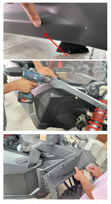
5. There is a fixed point at the rear of the fender flare, but since the original vehicle has no positioning point here, it is necessary to drill holes with a drill (3mm) according to the screw holes on the fender flare, and then fix it with screws.
