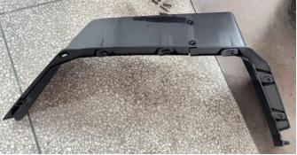
4. There are 8 positioning points on the flying wing decorative panels on both sides of the front of the original vehicle. Use a 3mm drill to drill out screw holes, and then install the assembled fender flares on the original vehicle with screws.
