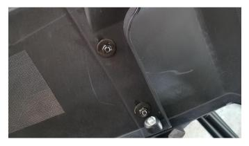
3. Install the fender flare on the vehicle by 5X30 self-tapping screws and flat washers.
