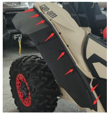
4. Attach the two ends (as the arrows show) to the vehicle by M5X20 screws and M5 nuts.
