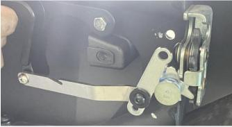
7. Snap on the spring in the same way as the picture. (The other side of the door handle is installed according to the above steps)
