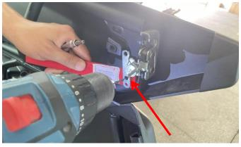
4. Assemble the new door handle, the first stainless steel bracket with screws fixed in the handle (bracket needs to determine the direction, the screws first do not screw too tight).
