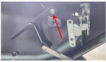
6. Use the screws to fix the stainless steel bracket with the original vehicle locking bracket together.
