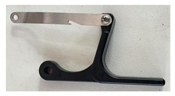
5. Snap the steel card from the product kit to the original vehicle's handle bracket. Then fix the screws on the steel card as shown in the picture.
