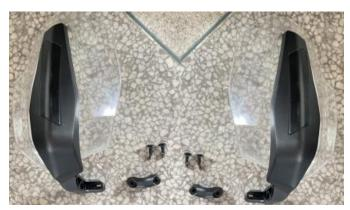
3. First install the handguard on the handlebar of the original vehicle, adjust the angle and then fix it with screws.
