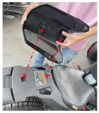
3. Press hard on the end of the decorative plate until you hear the snap sound, then screw on the fixed valve from the bottom of the shelf.
