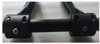
4. Fix the spare tire rack on the rear frame with four M8\*70 inner hexagon screws, four M8 flat pads and four M8 locknuts.
