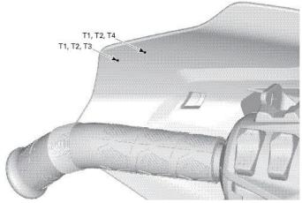
**Notice:** Make sure to drill perpendicular to deflector surface and make sure drill bit does not shift during operation.
