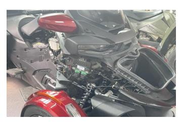
4. Remove the center fairing bracket from the original vehicle, then snap the fairing with lights onto the center bracket. Turn the fairing back to its original position after the installation is completed.
