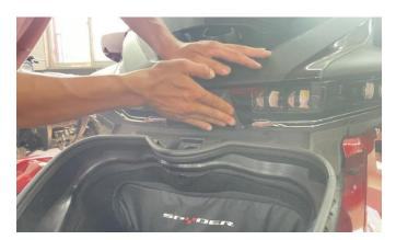
5. Disconnect the original daytime running light harness plug-in, use the adapter cable that comes with the product to dock with its plug-in, and dock the other end to the original vehicle socket. Pull the extension cable to the center fairing and connect it to the light harness. Finally, install back the previously removed accessories and decorative plates.
