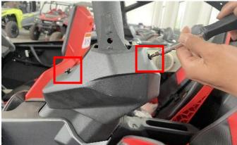
5. Snap the small guard plate on the large guard plate and fix it with screws.
