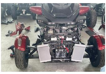
5. Remove the filter and air intake trim on the front bumper from the storage compartment. Remove the storage box and disconnect all wiring harness inserts inside.
