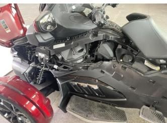
4. Remove the original front storage box and front bumper, disconnect the connecting harness plug.
