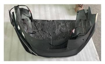
6. Remove the baffle of the original vehicle's daytime running lights on the front bumper, and then install the daytime running lights. Carry out the wiring work of the transfer line in the order shown in the figure, and connect the daytime running lights in sequence.
