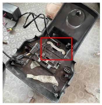
4. Dock the license plate light harness with the original harness, and sort out the excess harness according to the alignment of the original license plate light harness. Then start the car and check whether the license plate light can work properly. Finally, install the license plate light mounting shell and fender back to the original vehicle.
