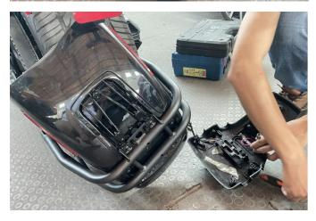
3. As shown in the figure, screw off the 2 nuts on the rear shell of the license lamp before installation, and put the license lamp behind the installation shell; Then, put the pressure plate removed from the original vehicle onto the screws of the rear housing of the license lamp from the reverse side of the mounting housing, and finally screw on the nuts.
