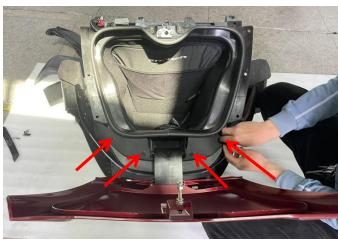
5. Use one end of the matching adapter cable to connect the LED auxiliary light harness plug-in, clip other adapter cables into the trunking on the storage box, fix the storage box on the front bar with the previously removed buckle, and install the grille and other decorative panels.
