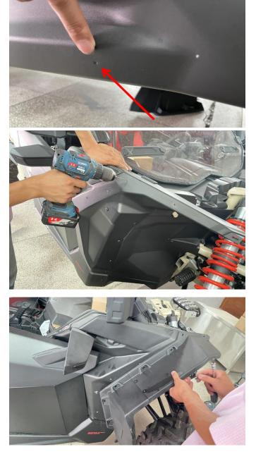
5. There is a fixed point at the rear of the fender flare, but since the original vehicle has no positioning point here, it is necessary to drill holes with a drill (3mm) according to the screw holes on the fender flare, and then fix it with screws.
