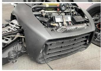
6. Connect the extension line with the harness of the accent light, install the front bumper on the fairing, and then fix it with the original screws of the vehicle.
