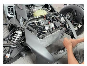
5. Disconnect the wiring harness plug-in, take out the conversion cable attached in the product, and then reconnect according to the corresponding plug-in, and then pull the extension cable through the gap of the vehicle to the front radiator and out of the cowl grille.
