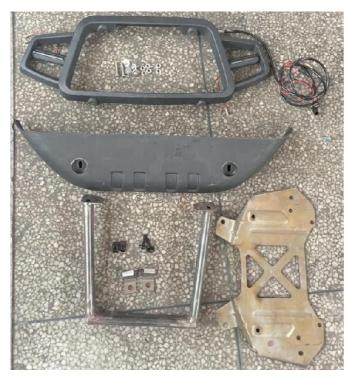
3. Fix the frame of the front bumper and the chassis with screws, and then install the front bumper and the lower protector on the frame.
