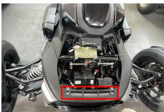
5. Before installing the lamp, you need to drill the screw holes in the vehicle with a pistol to facilitate the fixing of the lamp.
