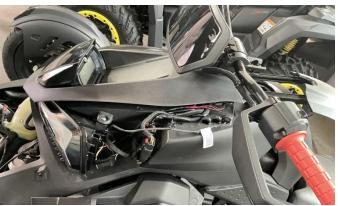
8. Find the location of the headers shown in the diagram, unplug the original wiring harness plug, and use the provided adapter cable to connect to the corresponding jack.
