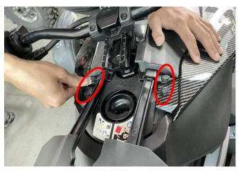
7. As shown in the diagram, remove the sub button on the side of the cover trim panel.
