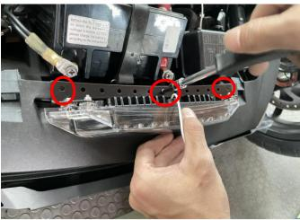
6. After the installation of the lamps is complete, you need to remove the decorative plate next to the front of the car, and then remove the logo in the picture 4 sub button.
