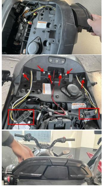
6. There is a gold resistor on the tail light wiring harness. The resistor needs to be installed on the bracket (the bracket is not divided into left and right), and then fixed with steel clips beside the screws on both sides of the car seat cushion. After completion, the seat cushion can be installed.
