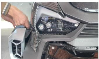
4. On the other side, you need to unscrew the 2 screws under the air inlet, remove the cover, and snap the decorative piece with the filter, after installing it, buckle the cover back and screw on the screw (there is a steel clip at the inner end of the cover, and The card slots in the same position of the vehicle body correspond to each other, so when installing the cover, install the front end first, and then the rear end).
