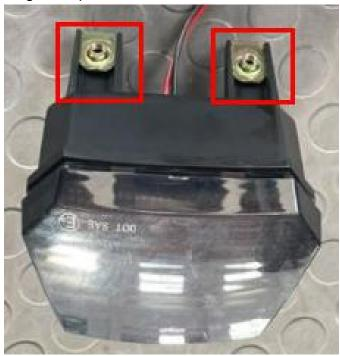
4. First remove the rear cushion, find the original tail light harness, disconnect the plug-in, remove the original tail light, install the new tail light, fix it with screws, and then connect the harness plug-in (you can start the car first to see if the tail light can be powered on properly and work)
