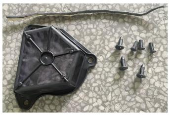
3. First take off the original vehicle after the air inlet cover, after placing the filter, in accordance with the screw holes on the filter, using an 8MM drill bit to punch three fixed holes after taking off the filter placed on the side of the spare, playing a good hole in the air inlet cover and then installed back on the original car (when installing the air inlet cover note that the edges have a bayonet, you need to correspond well with the slot on the vehicle body).
