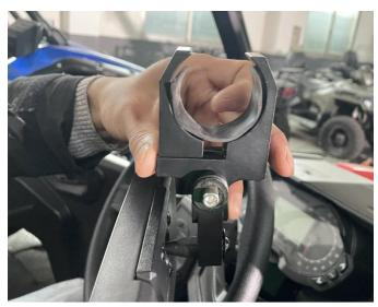
4. Clamp the reversing mirror on the front cross member of the original vehicle, and tighten it with the previously unscrewed screws. (Note: The interior mirror can be manually adjusted up and down to the desired angle)
