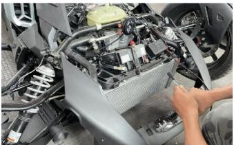
5. Install the front bumper on the fairing, and then fix it with the original screws of the vehicle.
