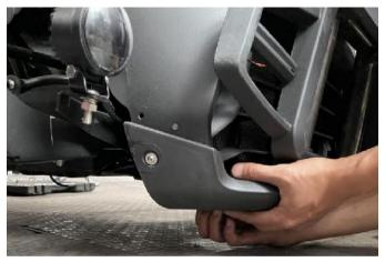
6. Clamp the steel clips in the accessory package on the two brackets shown in the figure, install the brackets on the bottom chassis of the front bar frame (one on each side), fix them with screws, and finally reinstall the engine cover.
