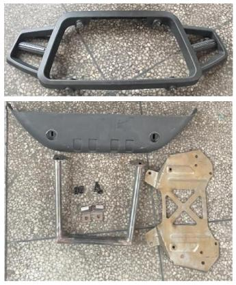
3. Fix the frame of the front bumper and the chassis with screws, and then install the front bumper and the lower protector on the frame.
