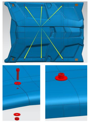
5. Stick the gasket with adhesive on both sides to the gasket plate. Keep the location clean before sticking.
