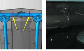
10. Attach the jockey clamp to the frame with 6x16 self-tapping screws. Also tighten all the screws in step 7, step 8 and step 9.
