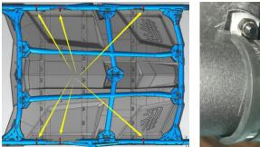
9. Use self-tapping screws 6x16 to mount the clamp on the frame, the screws are not tightened first.
