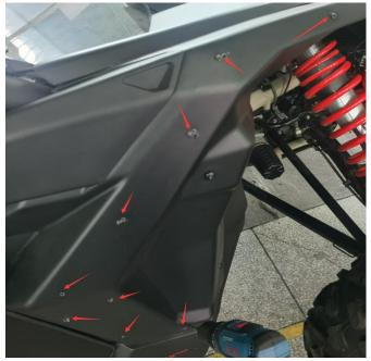
3. Remove the screws from the original car and spare.
