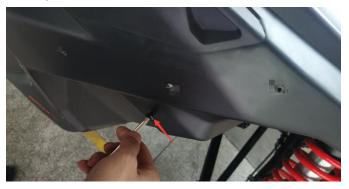
4. Install the screws removed in step3 through the holes indicated by the arrows on the widened front fender flare.
