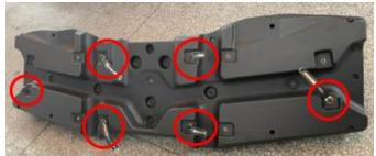
4. After installing the hoop, the audio bracket can be installed on the roof skeleton, and then use the hoop to wrap the skeleton with screws to fix.
