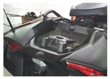
4. Keep the switch valve in the unlocked state, install the rear rack, lock the valve switch (the switch valve needs to be aligned with the valve port on the vehicle during installation), and finally hold the triggers at the bottom of both sides of the rack.
