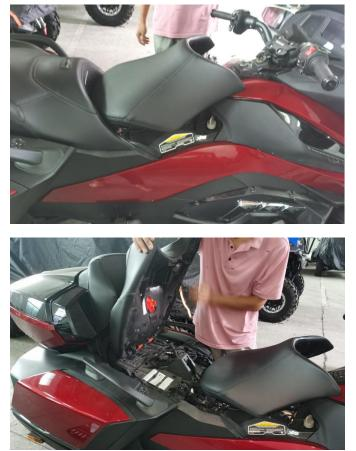
3. Open the rear cargo box, adjust the switch valve to the unlocked state, pull the trigger under the cargo box by hand, and finally remove the rear cargo box.
