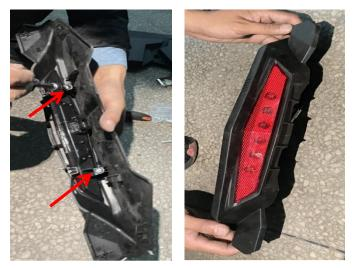
4. Put the bracket with the new taillight back on the vehicle, then reconnect the harness plug, and finally fix the taillight bracket with new extractor rivets.
