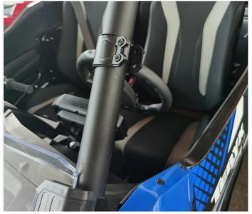
5. Install the mirror on the bracket by M6X45 screws.
