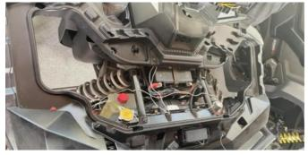
3. Unplug the wire harness plug-in of the central grid lamp, connect the wire harness to the headlight wire harness, connect the black wire to the black wire, and the gray wire to the green wire. After the wiring is completed, take insulation measures and spare.
