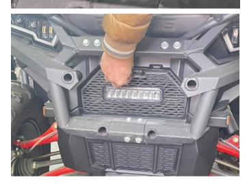
5. After the central network lamp is installed, insert the wire harness plug-in on the central network lamp and the plug-in that has just been paralleled to the wiring harness of the whole car (you can start the car first to check whether the central network lamp is normally energized), and then put it back in the storage Box, buckle the cover of the front guardrail.
