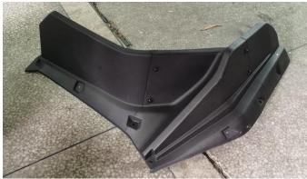
2. Remove the original fender flares and install the new fender flares.
