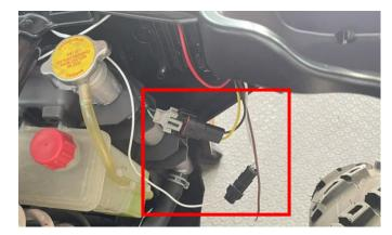
9. After the wiring harness is connected, start the vehicle first, check whether the headlights can work normally, no problem, you can put back the parts removed before, the installation is complete.
