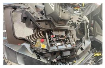
5. Take out the storage box, and then remove a crossbeam bracket in front of the vehicle to facilitate the removal of the original lights.
