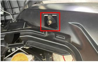
7. Install the new headlights and fix them with the springs and screws that were removed before (the headlights on the other side can be installed in the same way).
