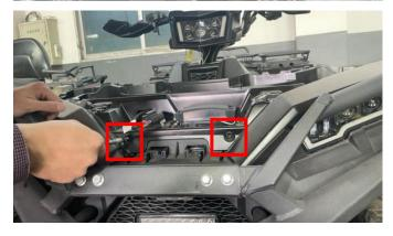
6. First remove the screws securing the original headlight, disconnect the headlight harness plug-in and take out the headlight (remove the spring and put it aside for backup).
