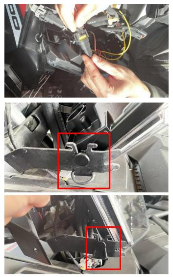
4. Open the buckle of the cargo box on the front of the vehicle, find the two on-off valves identified and screw them in the opposite direction, and take out the storage box.
