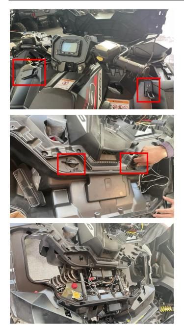
5. Open the cover of the ACC electrical box, take the white extension cord that comes with the product, peel off the outer skin of one end, and connect the marked wiring port with a copper wire.
