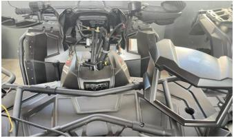
3. As shown in the picture, replace the new high beam headlights, wiring harness plug-in and the original vehicle docking good, fixed headlights at the bracket, both sides will be left with O-rings, the new headlights installed, you need to use the O-ring set on the headlights.
