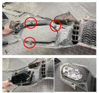
6.Pass the patch cord mentioned in above step 2 through the gap, pull it to the position of the headlight, and connect it with the plug-in on the headlight. After completion, start the vehicle and test whether the headlight can be powered on normally (the headlight on the other side can be completed as above steps 4-6), as shown in the figure:
