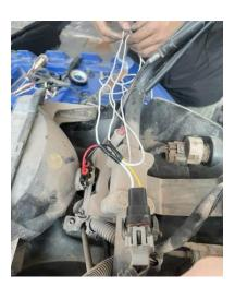
2.Remove the front bumper and original lights, and remove the plug-in of light wiring harness, as shown in the picture:
