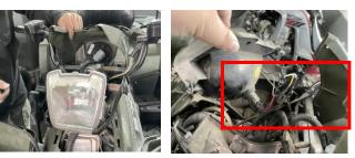
3.Remove the front bumper as shown in the picture:
