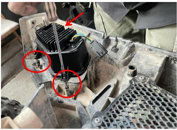
4.Pass the patch cord which connected on the high beam through the gap, pull it to the position of the headlight, and connect it with the plug-in on the headlight. After completion, start the vehicle and test whether the headlight can be powered on normally (the headlight on the other side can be completed as above steps 2-4), as shown in the figure:
