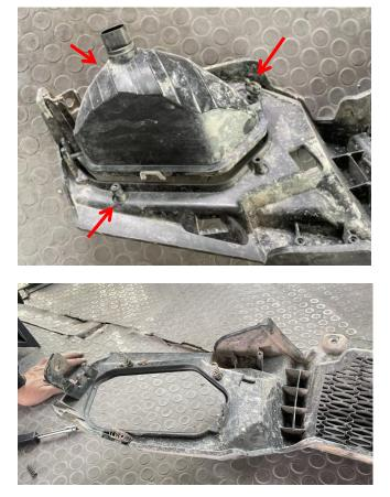
5.Set springs on the three screws which fix ed the headlights, install the new headlights as the orientation and fix them with screws, as shown in the figure:
