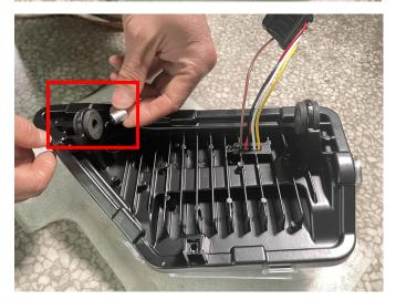
6. Install the headlights (accessories has been installed already) on the bracket in the same way that the original headlights were fixed, and connect the wiring harness plug-ins well, (the headlights come with steering function, you can wire as you need). Start the vehicle at the same time to check whether the headlights are turned on normally. As shown in picture:
