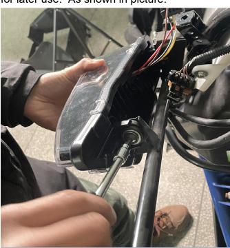
5. Clamp the round rubber ring of the original headlight accessories to the back shell bracket of the new headlight, and then thread the aluminum tube into the rubber ring. As shown in picture:
