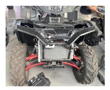
2. Remove the original headlights on the front bumper, and install the new headlights as the original headlights (use the accessories of the original vehicle or the new product), and the headlights on both sides can be installed in the same way. As shown in picture:
