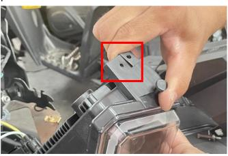
3. Start the vehicle and turn on the switch of high beam, to check whether the high beam can be turned on normally. When finished, you can fix the headlight and re-fasten the rubber rings and adjusting screws on both sides of the headlight. As shown in picture:
