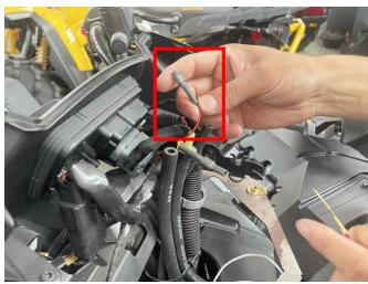
2. Disconnect the wiring harness plug-in, remove the original headlight, pry the steel clip on the original headlight with a tool, and clamp it on the new headlight according to the original position. Take out the patch cord of the product, connect one end with the original vehicle wiring harness, connect the other end with the new headlight, and connect the remaining red extension wire with the original vehicle reserved wiring harness (red). As shown in picture:
