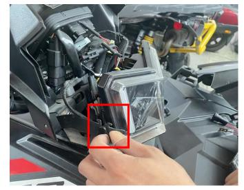
4. Install back the decoration cover of high-beam headlight, as shown in the picture:
